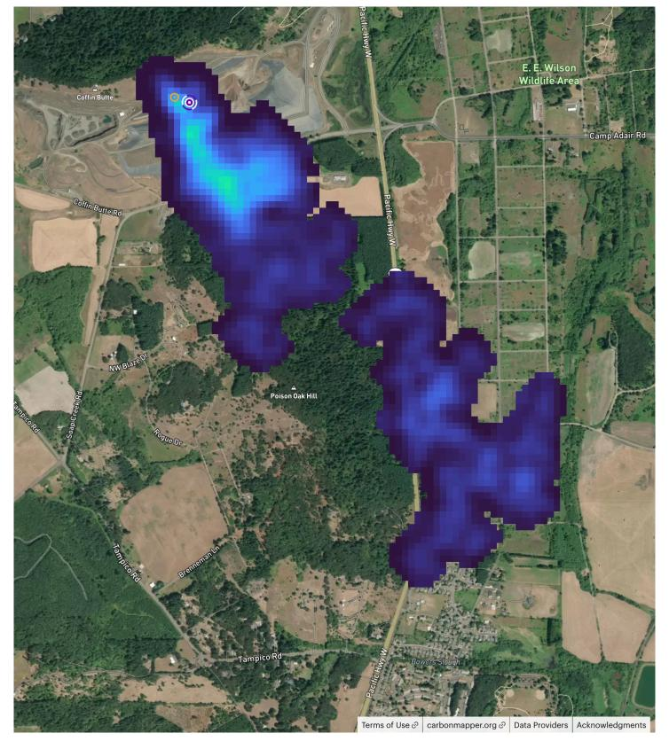
The methane plume is of course the blue-to-green blob stretching from upper left to lower right of this image. The methane detection technology employed here looks for methane at superemissions levels – i.e., from a point source that's emitting more than 0.1 metric tons of methane per hour. Analyzing the data for this particular plume results in a leak rate of 1.2 metric tons of
